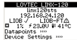
Figure 30: Main Screen of the LCD UI.
