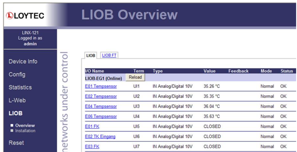
Figure 12: Test L-IOB inputs and outputs on the Web UI.
