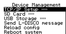
Figure 31: Device Management Menu on the LCD UI.
