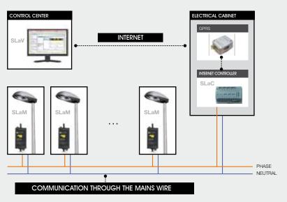
The *SLaM-ON* device uses the existing mains wire to communicate up to the control cabinet. The cabinet includes the SLaC Internet Controller and a GPRS modem to communicate up to the maintenance center, where the SLaV software application informs about the luminaires status and alarms.
