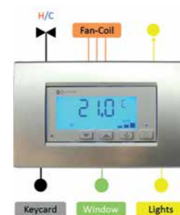
2 pipe system + keycard occupancy control
