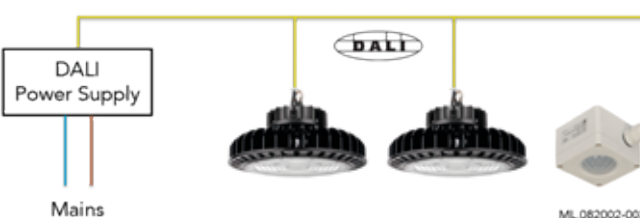
Solution with integrated CLC in Multilux High Bay DALI Master
