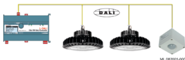
Solution with DALI Controller and LonWorks multisensor
