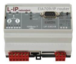
An L-IP redundant CEA-709/IP router can be used as a single device to achieve redundancy on the CEA-709 (TP/FT-10) channel by building a ring structure. If IT network redundancy is available, full redundancy on the IP-channel and on the CEA-709 channel can be achieved with two devices installed in parallel. In this case device redundancy is ensured as well by mutual monitoring of paired L-IP redundant routers.
