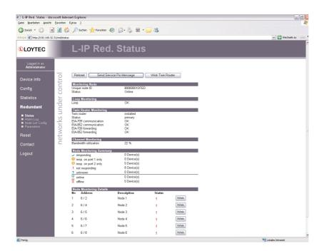
Without using an LNS plug-in the L-IP redundant CEA-709/IP router can be configured via the built-in web server, which also shows the health status of the TP/FT-10 ring and the connected nodes.
